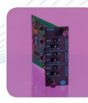
The V3/04 is a 3 channel interface for use with triaxial voltage (IEPE) accelerometers. Inputs to the V3/04 can be via a 3 standard Microdot The V3/04 is a three channel interface, for connectors or 4J, 4 way single input connector from the AT Series accelerometer. Each channel provides switchable gain over the range x1, x3.16, x10, x31.6, x100 = 40dB, 10dB steps Gain
